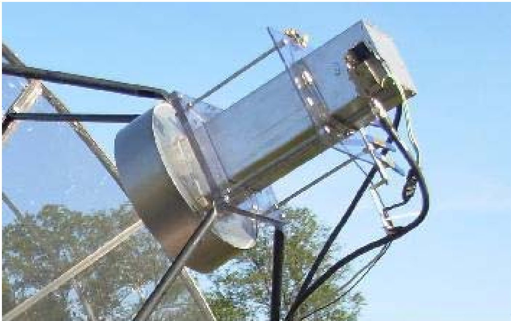
Figure 1 Septum feed with choke ring (from WA5WCP)
