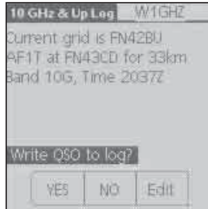
Fig 5—Once the band is selected, the entry information is displayed for confirmation before it is stored.
