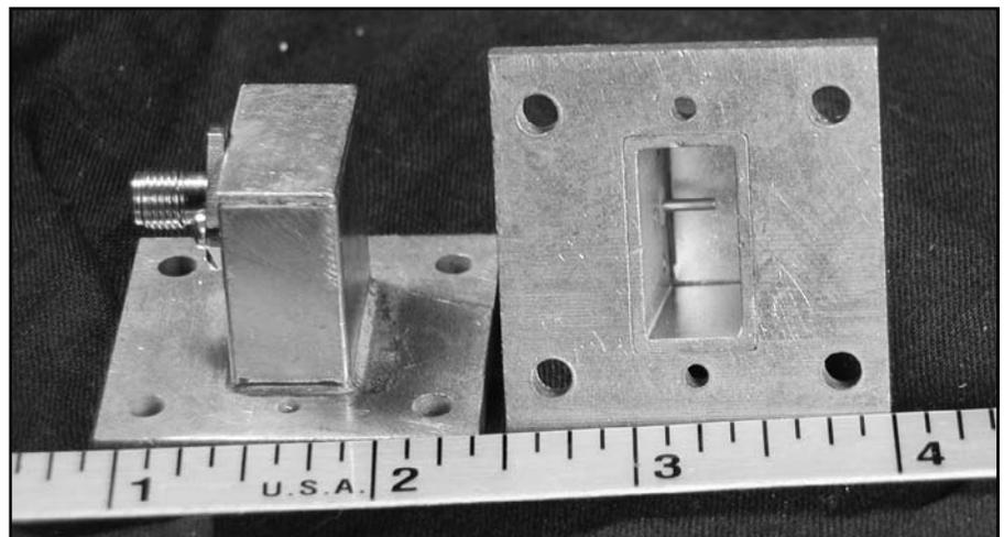
Figure 1 — WR-75 waveguide to coax transition for 10 GHz.
