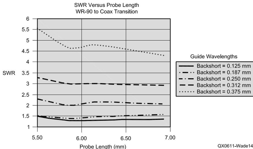
Figure 14 — WR-90 to coax transition, SWR versus probe length at 10.368 GHz.
