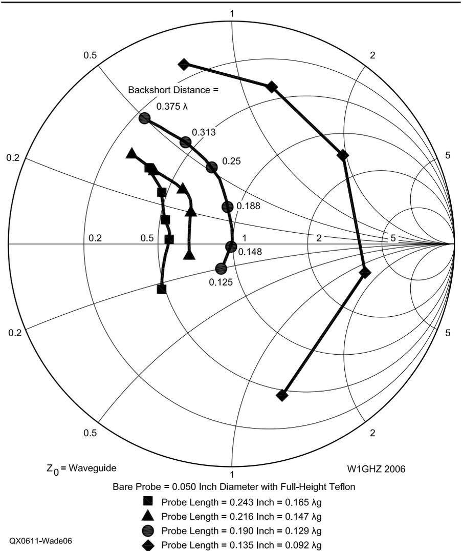
Figure 6 — Smith Chart plot of impedance as dimensions are adjusted for WR-90 to coax transition with full height Teflon.
