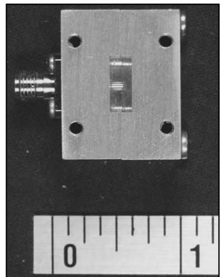
Figure 15 — WR-42 to coax transition for 24 GHz in milled aluminum block.
