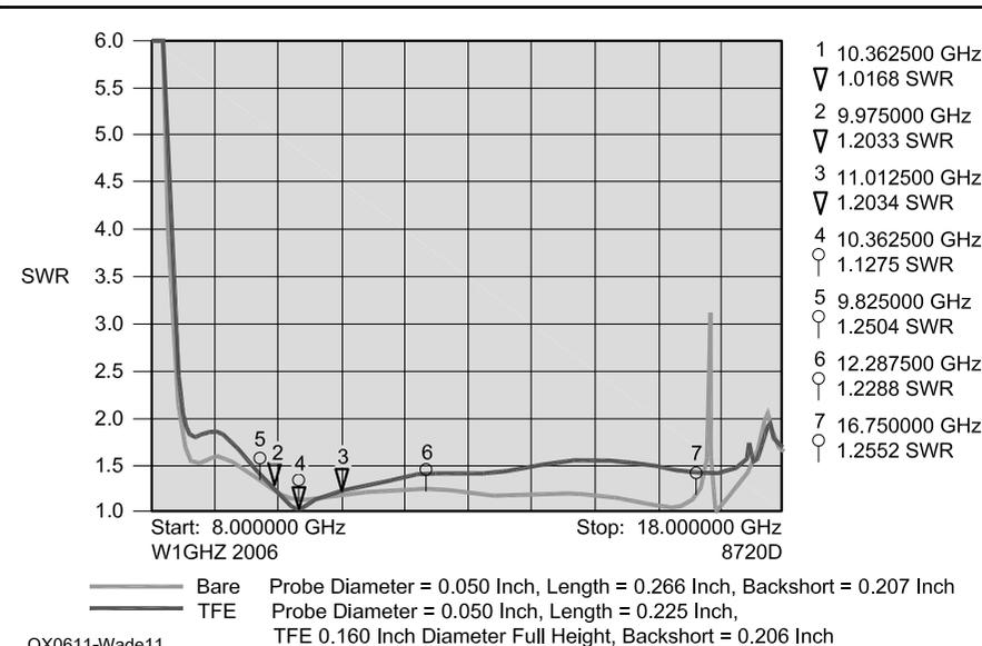
Figure 11 — SWR versus frequency of WR-75 to coax transition.
