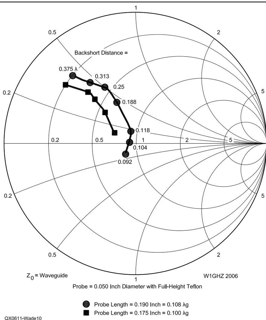
Figure 10 — Smith Chart plot of impedance as dimensions are adjusted for WR-75 to coax transition with full height Teflon.
