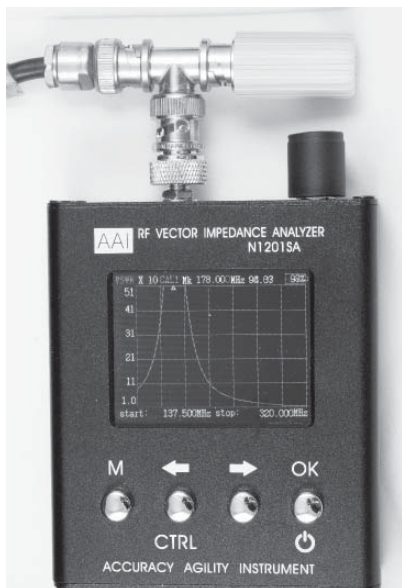
Figure 8 — Measuring resonant frequency of a stub
